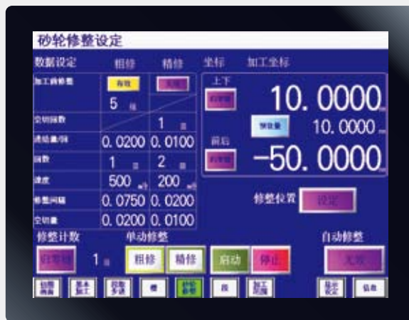
自动修砂条件设定画面 自动修砂条件粗/精加工可分别进行设定。 Setting the dressing conditions for Rough and Finish Rough and Finish dressing can be set separately.
