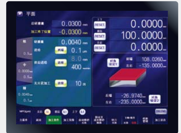
档案功能 Recipe 保存·读取加工和砂轮修整条件 Grinding data and dressing data can be saved screen.
