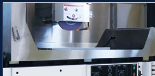
加大了工作台前部的开口，从而达到轻松装卸工件 Wide cover realized easy workpiece detaching.
