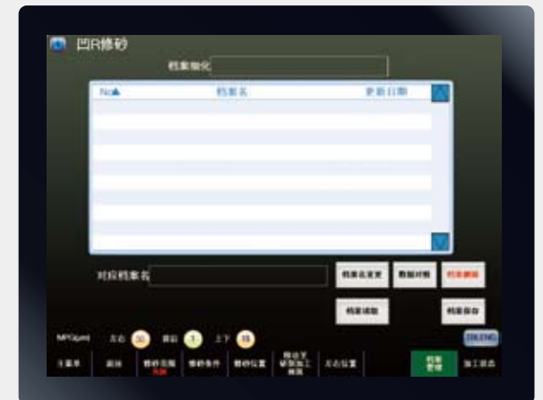
档案功能 Recipe 保存·读取加工和砂轮修整条件 Grinding data and dressing data can be saved screen.
